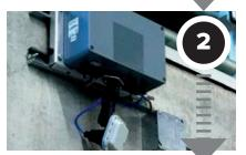
Receivers mounted permanently between the upper and lower decks of the stadium read signals from all players on the field pinpointing a players' position, tracking speed, acceleration, and distance traveled in real-time.
