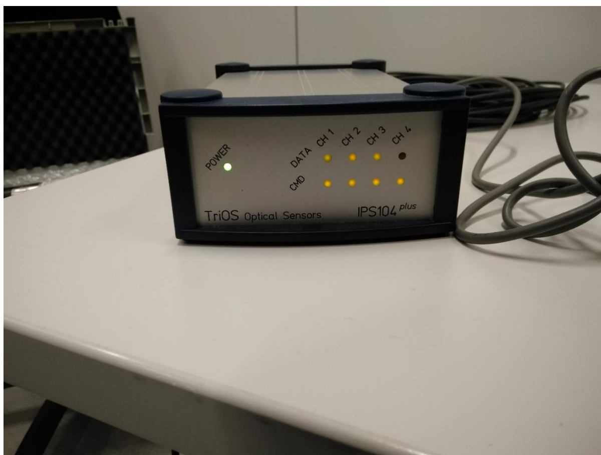
Figure 6 IPS104 box showing lights when 3 radiometers are connected. Top row lights flash brighter when data is being acquired.
