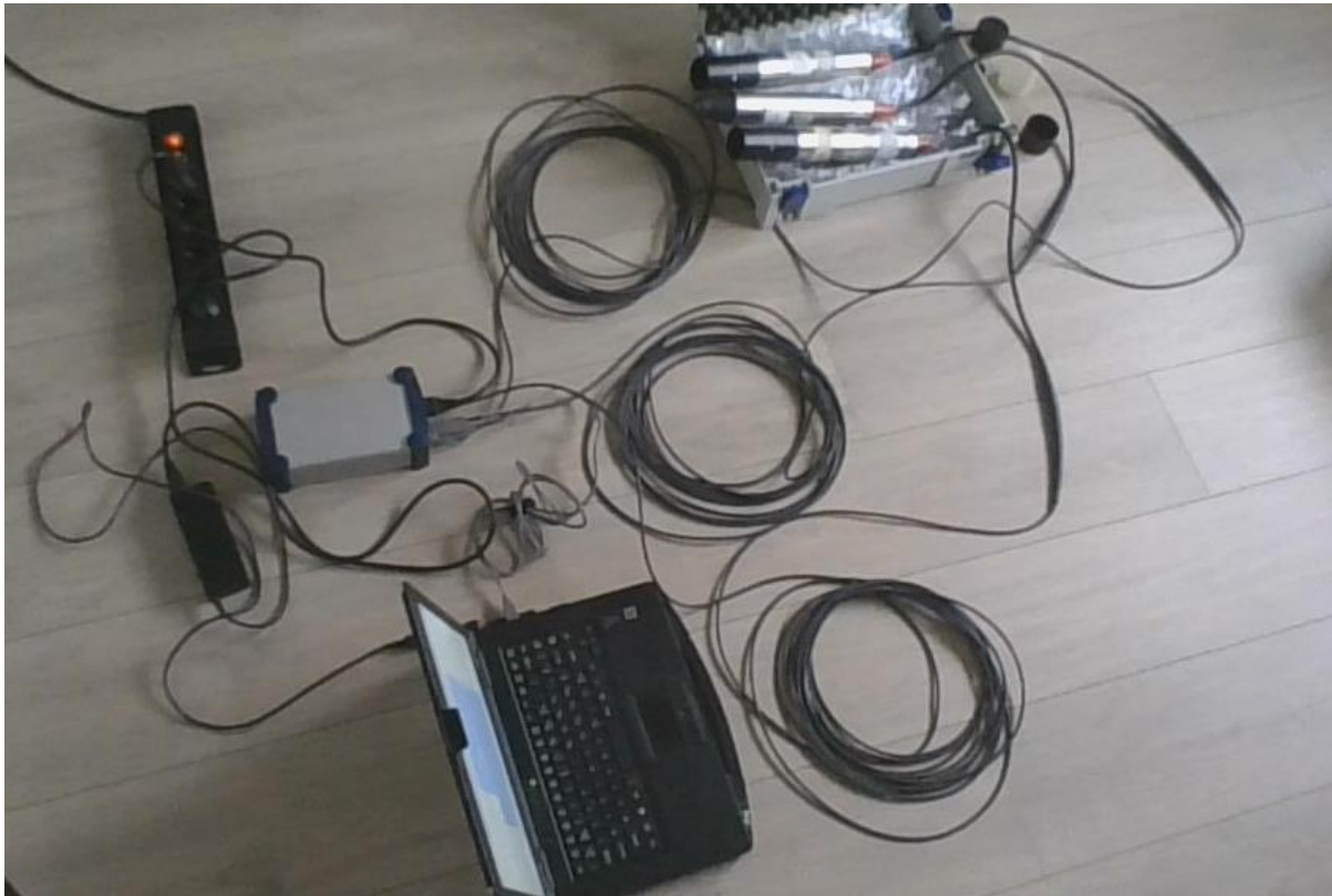
Figure 3 Radiometer measurement system consisting of (from left to right): Multi-socket power board, IPS104 radiometer power supply and data interface box, acquisition PC, RS23/USB adapter grey cable, 3*50m SUBCON/M8F RAMSES cables, box with one irradiance and two radiance TRIOS/RAMSES sensors and dummy connectors and lens caps. No external GPS is shown here since the PC internal GPS is used.
