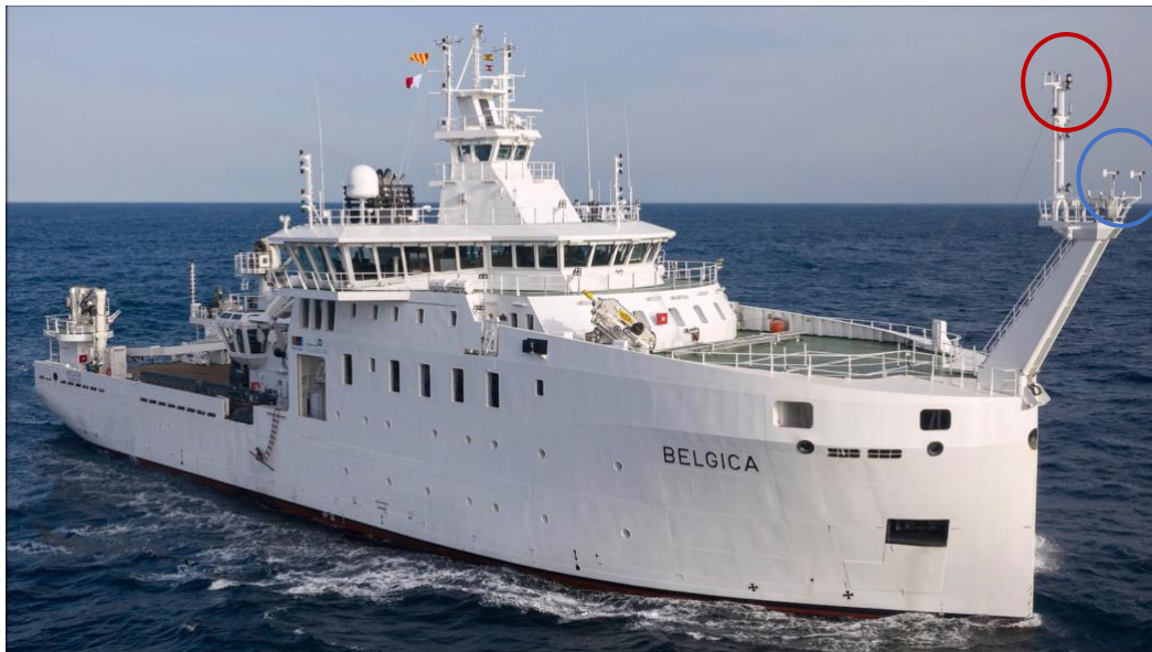
Figure 2 Good locations for installation of abovewater radiometer system on the new Research Vessel Belgica-2. The blue circle shows the optimal location (prow facing-forward) for radiance measurements to avoid optical and hydrodynamic perturbations from the ship. The red circle shows an ideal location for downwelling irradiance measurements, although for safety reasons this may be inaccessible and the blue location may be a reasonable second choice.
