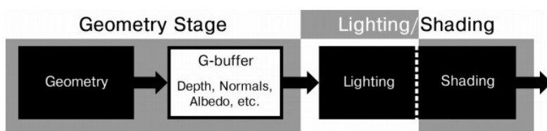
Figure 1: The stages used in deferred shading. The first stage renders several properties of the opaque geometry to the G-buffer. The G-buffer is used to calculate the lighting and shading, which can be done in a single stage or two separate stages.
