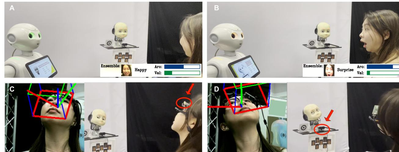
Experimental set-up within different conditions: A) The iCub mirroring facial expressions; B) The Pepper affectively signaling through LED color changes; C) The iCub mirroring head movement based on IMU readings. The red circle shows the IMU; D) The iCub mirroring head movement based on a vision-based model. The red circle shows the camera.
