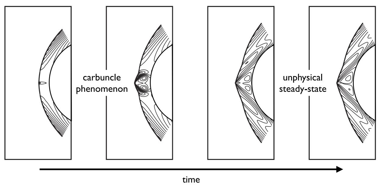
Mesh must be adapted to align with critical flow structures to maintain accuracy.
