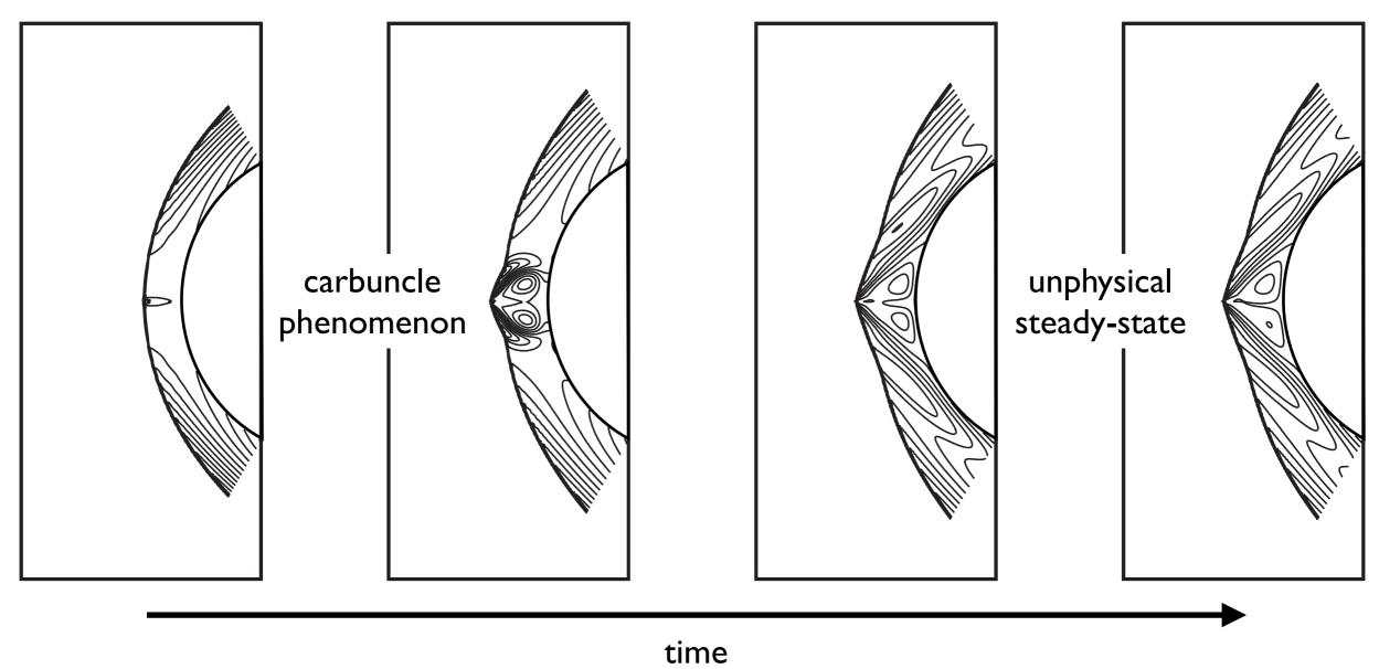
Solution accuracy depends on mesh alignment and resolution
