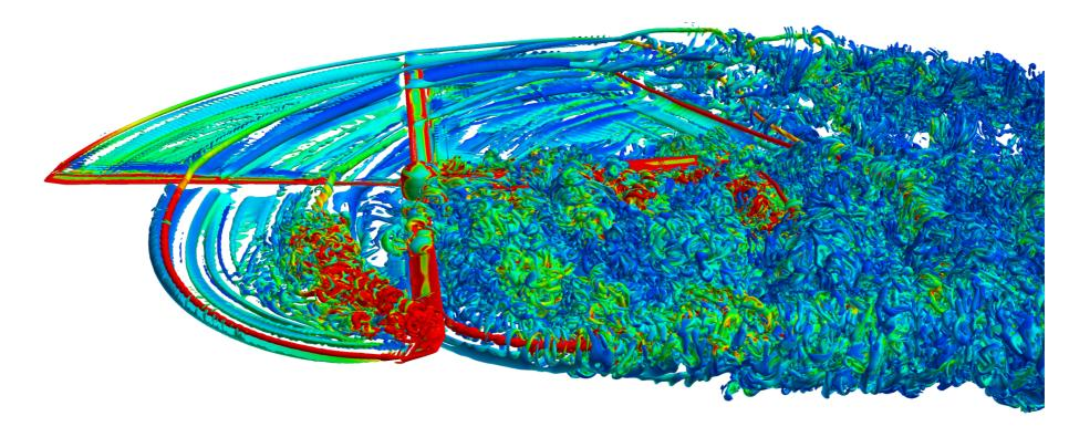
Simulation of dynamic stall for a Blackhawk helicopter rotor in forward flight. (credit: NASA ARC).
