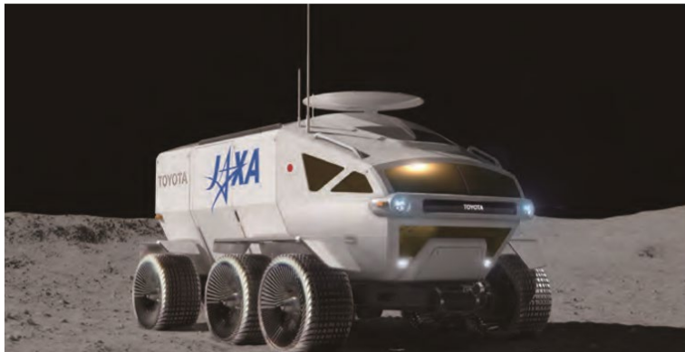
A mobility required for human exploration on lunar surfaces "Manned Pressurized Rover" (source: Toyota Motor Corporation)
