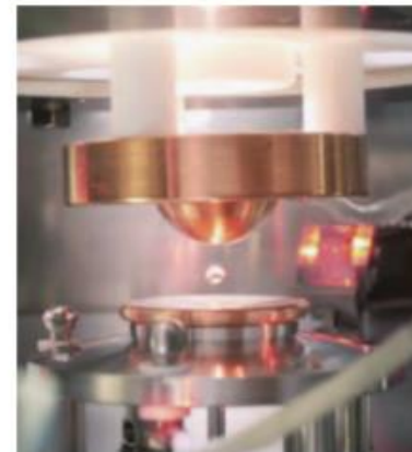
An experiment on the electrostatic levitation furnace on Earth: an electrically charged sample is levitating in electrostatic field generated by a voltage applied between the electrodes.
