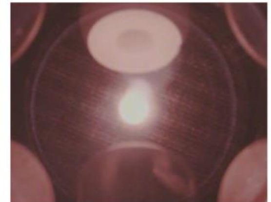
Molten aluminum oxide (central object) levitating between six electrodes (photo taken in July 2017)
