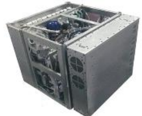
This picture shows a demonstration model for the next-generation water regeneration system, 1/4 in size compared with the current one.
