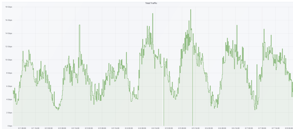
Figure 5: Tap Bandwidth — We deployed Conjure in a realistic ISP testbed on a tap of a 20 Gbps router. In a typical week, traffic ranges from 2–17 Gbps.
