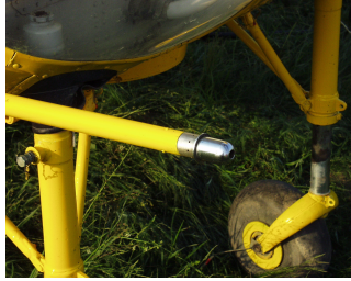
Exhibit 4: Pitot tube mounted on a helicopter (Zátonyi Sándor, en.wikipedia.org/wiki/Pitot_tube ) showing one large, forward-facing, circular orifice to measure total pressure, and several small circular orifices behind a trim ring, to measure static pressure.
