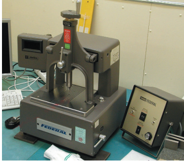
Exhibit 5: Version of the Mahr-Federal comparator model 130B-24 used by the Dimensional Metrology Group (Semiconductor and Dimensional Metrology Division, Physical Measurement Laboratory, NIST) for the mechanical comparison of dimensions of gauge blocks.
