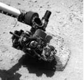
**LEFT** Curiosity isn't just driving around...we're doing science! This image shows the robotic arm of NASA's Mars rover Curiosity with the first rock touched by an instrument on the arm. The rover will use its drills, scoops, and various instruments to analyze the rocks and soil that it encounters.
