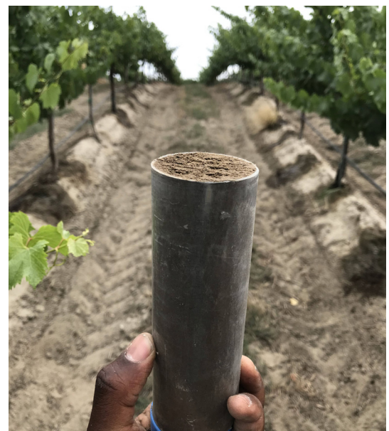
Figure 28. Soil scientists sampling soil bulk density in vineyards to quantify soil health. (Photo: Sarpong)
