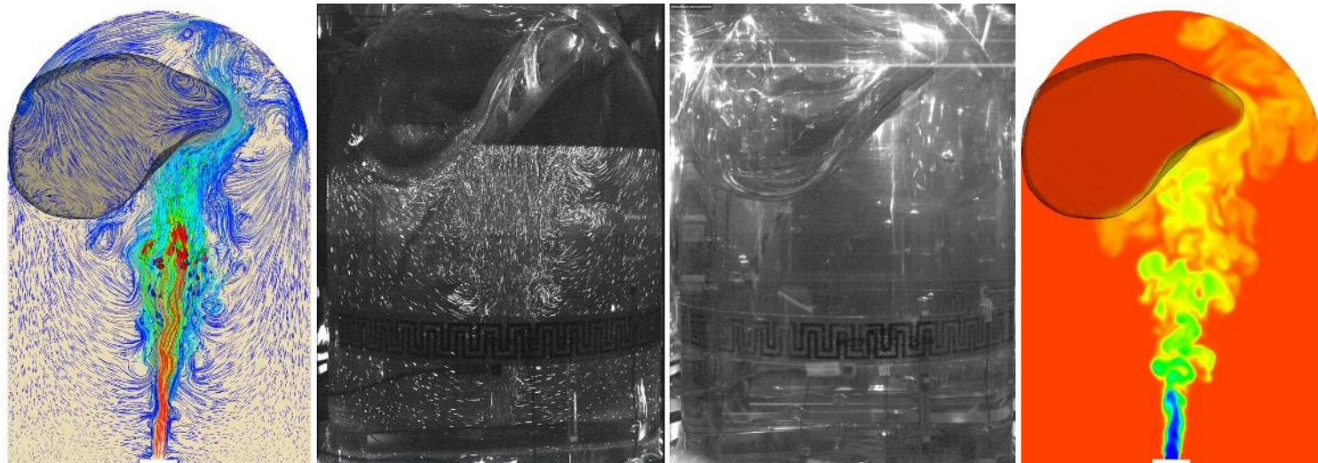
CFD Models predict fluid and thermal profile against ZBOT-1 data
