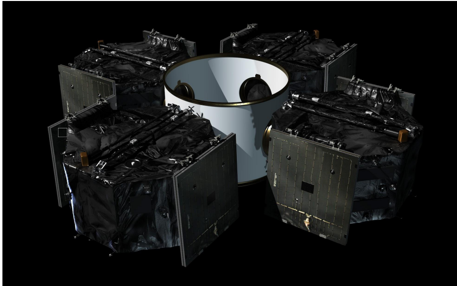
Figure 8-23. Rendering of four CREO spacecraft mounted on an ESPA Grande ring. The total span of all mounted spacecraft fits within a 4-m fairing.
