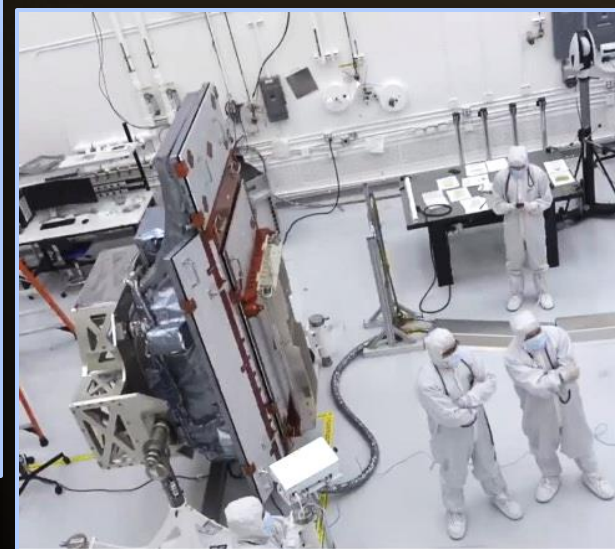
Roman WFI recently underwent vibration and acoustics testing and successfully completed its second and final thermal vacuum test in May.
