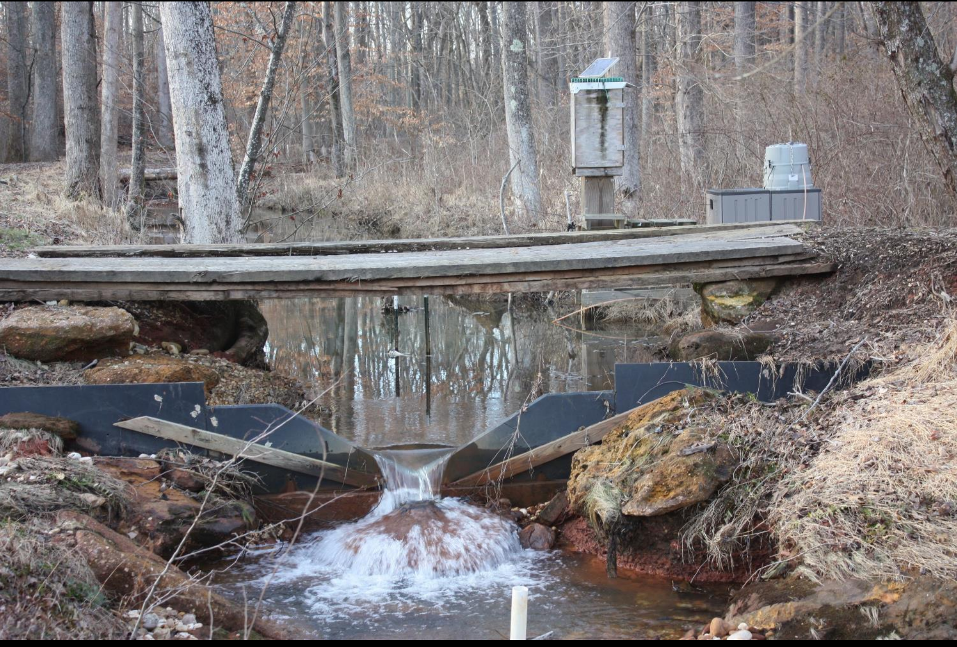
The weir and automated sampler at the outlet of the restored reach
