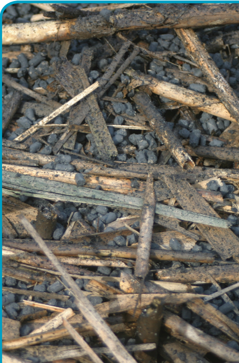
Pellets of activated carbon can absorb toxic mercury and methylmercury before they enter the water. (Credit: Upal Ghosh/University of Maryland)
