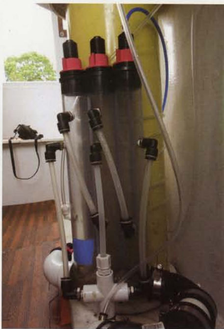
The CO 2 equilibrator above measures the concentration of CO 2 in the water. Its other half, an orange box that stores the data, is stashed in a cabinet in the Ault's galley.
