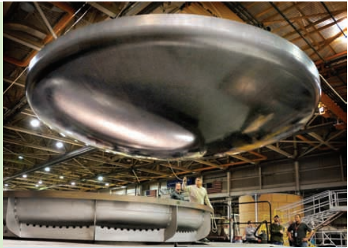
The Orion heat shield structure hovers above its layup mold during removal at the Lockheed Martin composite development facility. (Credit: Lockheed Martin)
