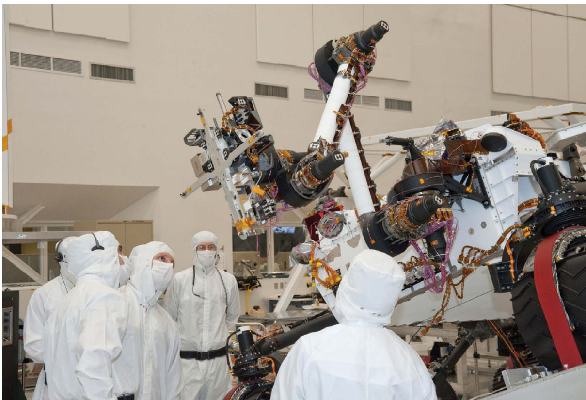
FIGURE 1.9 Mars Science Laboratory Curiosity rover undergoing a test of its sample arm while on a tilt table at the Jet Propulsion Laboratory in September 2010. SOURCE: NASA/JPL-Caltech.
