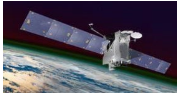
Photo Credit: NASA's Scientific Visualization Studio NASA's Global-scale Observations of the Limb and Disk (GOLD) instrument is hosted by a commercial communications satellite, operated by SES Government Solutions . GOLD is examining the response of the upper atmosphere to interactions with the Sun, magnetosphere, and the lower atmosphere.
