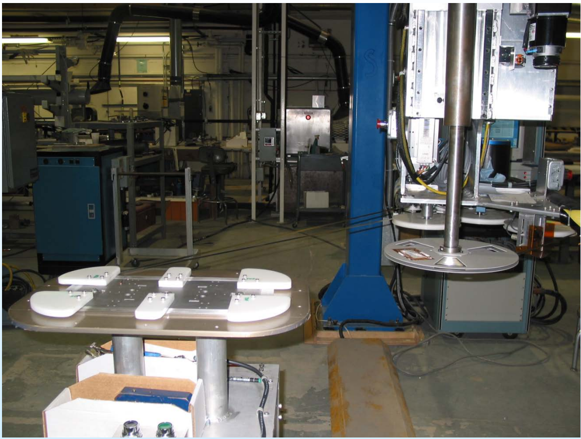
Modern computer controlled coil winding machine @BNL
