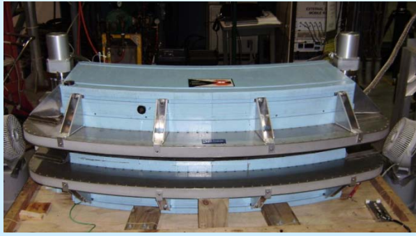
Cu coils replaced by cryo-cooled HTS coils by HTS-110
