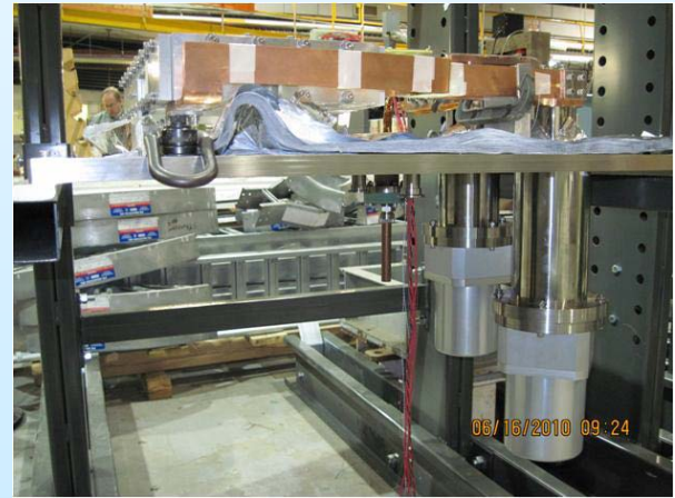
Cryo-cooled HTS coils with technology developed at BNL
