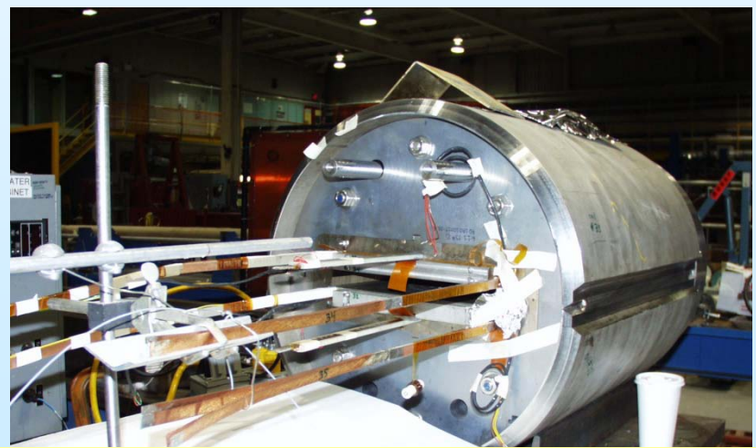
Record 10.4 T in R&W Nb 3 Sn Magnet
