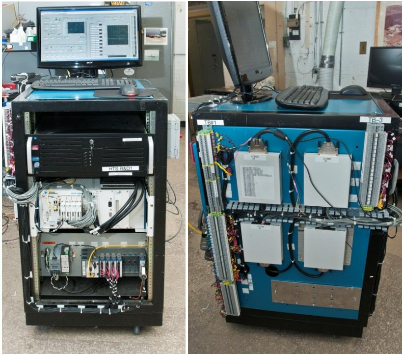
Cabinet #1 (32 channels, 1kV)
