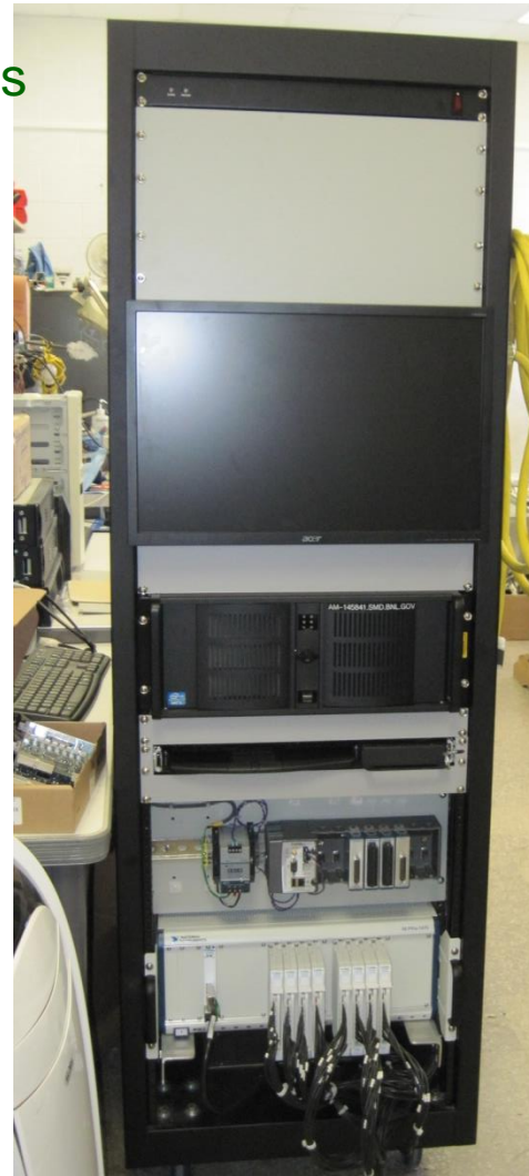
Cabinet #2 (32 channels, 1kV) (expandable to 64 and 3kV)
