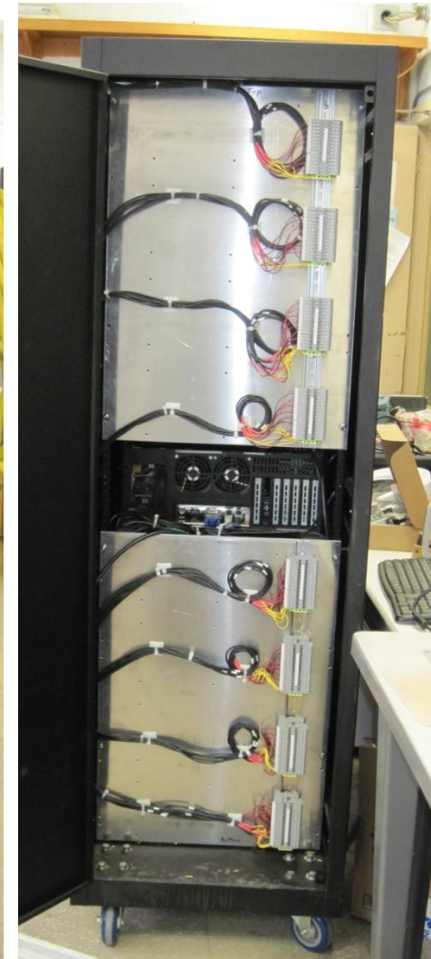
Cabinet #2 (32 channels, 1kV) (expandable to 64 and 3kV)
