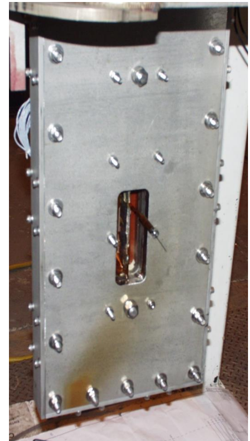
HTS Cable Coils in support structure
