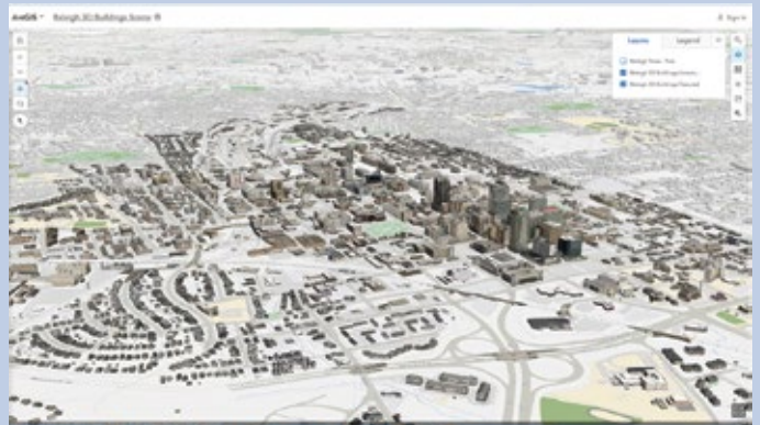
3D features were extracted from LiDAR Data to help create the 3D Basemap. This map became the foundation of the InVision Raleigh Application.
