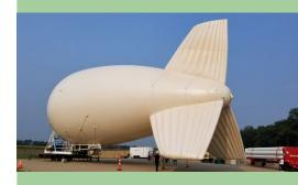
WHIN has also launched an aerostat—a blimp-like aircraft—in partnership with RTO Wireless to support WHIN's research broadband network. The aerostat, tethered between 1,500 and 2,500 feet, offers better lines of sight than land-based wireless towers, supporting both LoRaWAN and broadband coverage. The partnership with RTO Wireless, as well as other private tech partners, will allow WHIN to test innovative broadband solutions and eventually publish the results of those tests.
