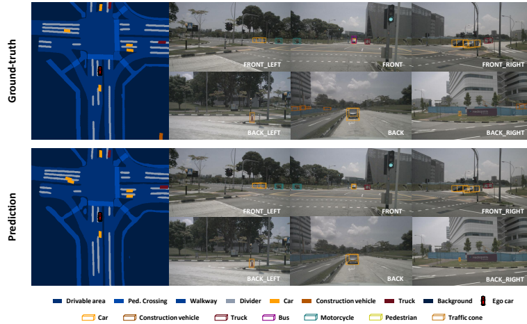
Fig. 5: Qualitative results on nuScenes dataset. Left is the BEV segmentation map with projected vehicle 3D bounding boxes result from detection head. Right are in image perspective with prediction results. Different colors stand for different categories.
