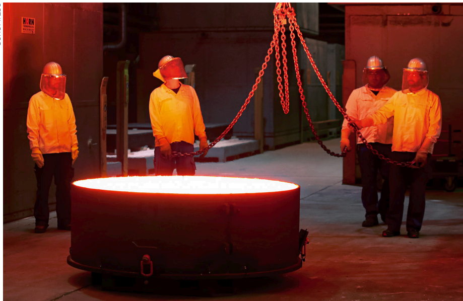
Figure 4. This image shows the first cast from which six blanks will be obtained by SCHOTT (Germany) at their facility in Mainz. This first cast is a thick cylinder that will be cut into six slices, each of which will become a segment blank.
