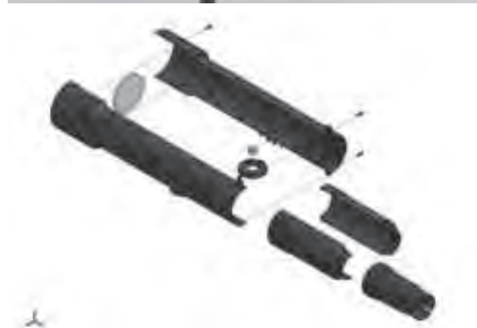
Fig. 3. Structure of new "You are Galileo!" telescope
