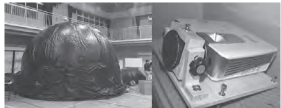
Fig. 1. Left: DIY inflatable dome, Right: Full HD projector with a fisheye conversion lens.
