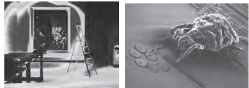
Fig 1. (a) Pseudo-colors representing the temperature (Infrared camera, false colors reported in greyscale); (b) Acarus close to a nanotech motor (Scanning electron microscope, greyscale).
