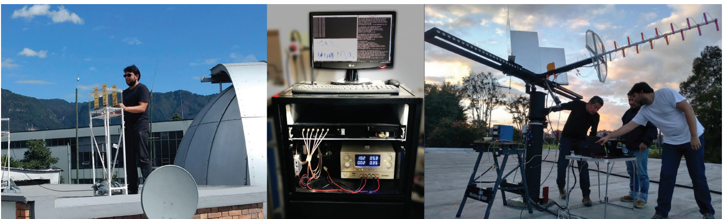
Figure 6. Radio interferometers installed on the terrace of the National Astronomical Observatory at Universidad Nacional de Colombia. The instruments have been developed by undergraduate and masters' students as part of their research projects. The First Colombian Radio-interferometer (FiCoRi) (see the acquisition system in the middle panel of the figure) represents an important milestone in the development of radio astronomy instrumentation in Colombia. Credit: From the digital archive of the National Astronomical Observatory of Colombia.
