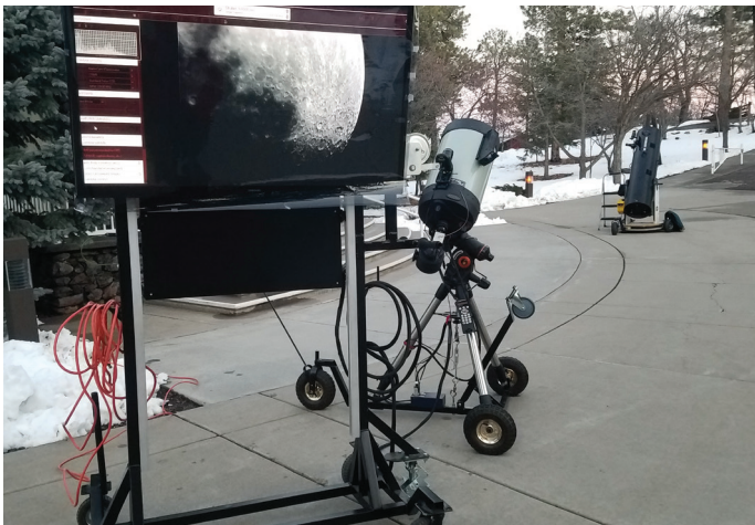
Figure 3. Our system incorporated an 11-inch Celestron telescope, a MallinCam Xterminator camera, and a large-screen television to display images directly to the public (left). We used live images from the telescope to entertain large crowds on busy evenings at Lowell Observatory and during our always popular 'Meet an Astronomer' evenings (right). Please note that the live television display of the Moon is overexposed in the right photograph, but clearly visible in the left. Credit: Sarah Burcher, Lowell Observatory (left); Jim Cole, Lowell Observatory (right)
