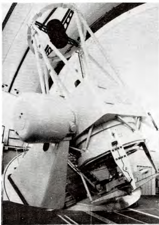
The 98-in Isaac Newton Telescope as arranged for direct Cassegrain photography
