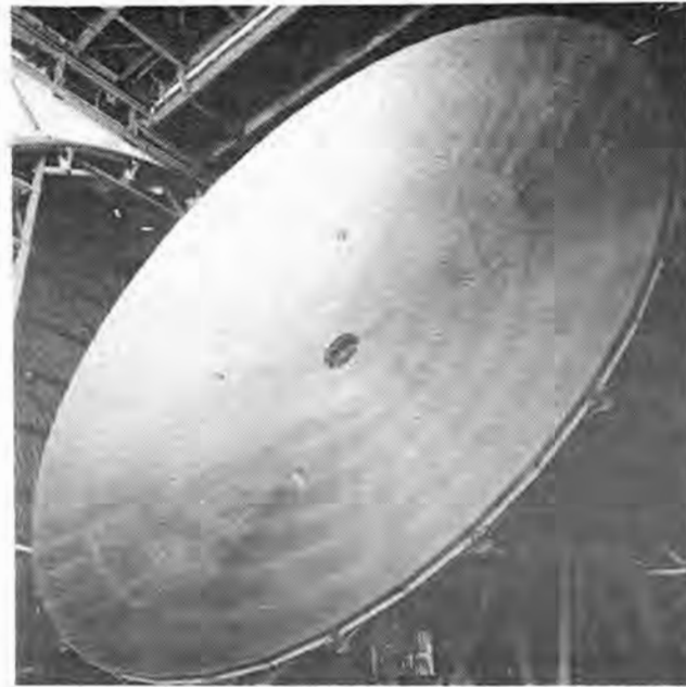
The 15-m primary mirror of the Maxwell Telescope. There are 276 panels in seven rings. Panels are accurate to about 12 micrometers (r.m.s.). Copyright 1987, Royal Observatory, Edinburgh.
