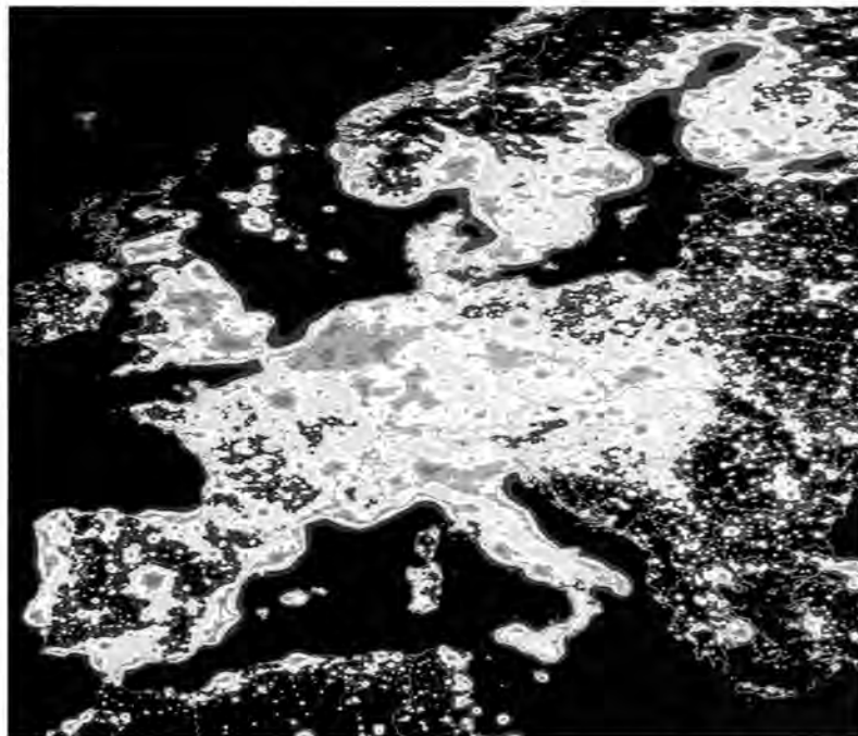
The artificial night sky brightness at the zenith in Europe in 1998/99 based on the upward flux measured by the U.S. Air Force DMSP satellite and on the modelling of the propagation of light pollution in the atmosphere.
