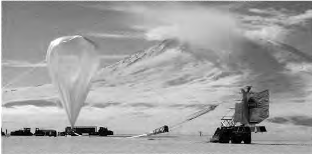
The BOOMERANG Telescope being readied for launch in Antarctica, with Mt. Erebus as a backdrop. The BOOMERANG Telescope made the first high resolution survey of the tiny 100ppm temperature variations in the cosmic microwave background.
