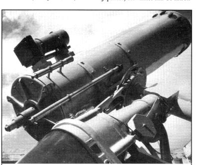
The 'Catts Telescope,' a nineteenth century instrument that somehow escaped Ian Glass's book on Grubb telescopes. During the 1950s and 1960s, this instrument was used at Mount Stromlo and Mount Bingar for a wide range of photometric and spectrophotometric studies by staff, visiting astronomers, and PhD students
