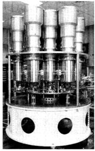
Above: The multibeam receiver for HICAT, used on the Parkes 64 m
