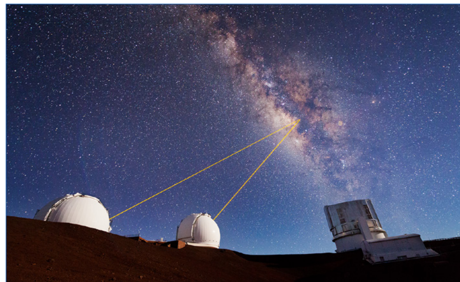
Both 10-meter telescopes of the W. M. Keck Observatory use their adaptive-optics lasers to study the supermassive black hole at the center of the Milky Way galaxy. [Sean Goebel / sgphotos.com ]
