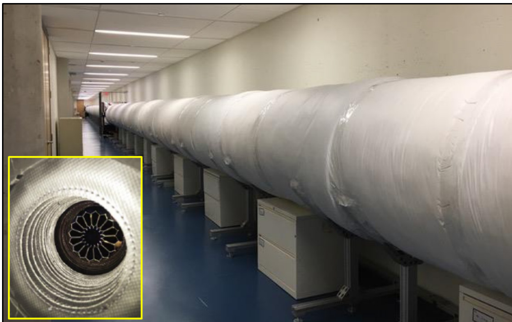
Figure 11.2-5. S5's starshade model validation testbed at Princeton. Model starshade shown in inset.
