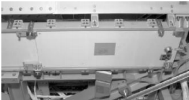
Figure 8.3-14. Left: ISS access hatches, sliding door. Right: Hinged lid (Harding 2011).
