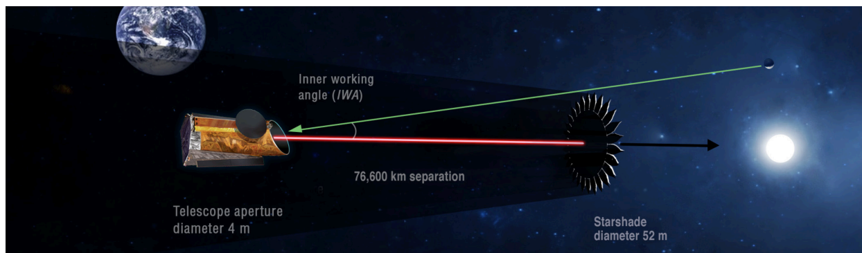
Figure ES-7. The HabEx telescope flying in formation with the starshade. The telescope can detect and characterize exoplanets viewable near or beyond the angular radius of the starshade as seen from the telescope, which defines the inner working angle (IWA).
