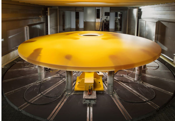
Figure 11.3-3. 4.2 meter European Extremely Large Telescope secondary mirror blank. Credit: SCHOTT.
