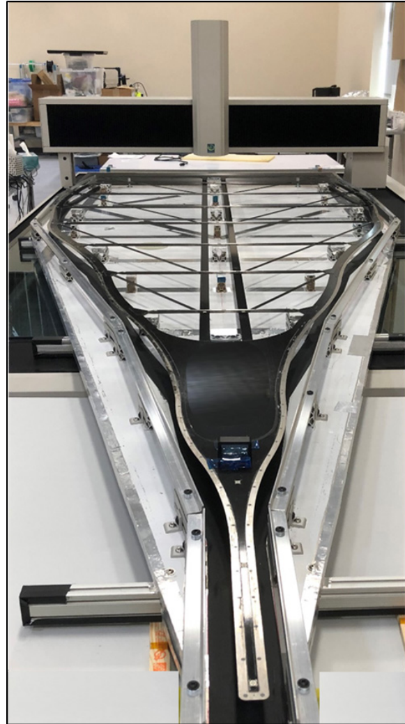
Figure 7.2-3. S5 Prototype 1 petal used to demonstrate shape accuracy after thermal and deploy cycles and to validate model of shape vs temperature (shape stability). Petal is sitting on Micro-Vu measurement machine at Tendeg's facility in Louisville, CO. The overhead optical head on gantry CMM is used to measure edge shape profile.
