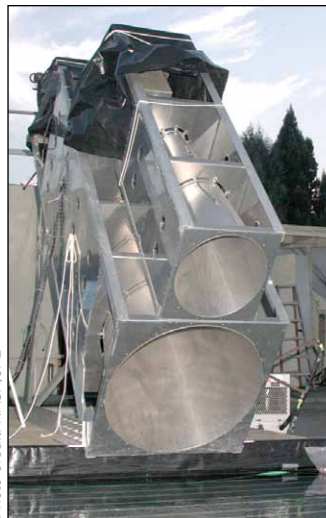
The Aquarius instrument prototype was used to test the mission's measurement principle by observing how 1.413 gigahertz microwave emissions responded to changes in salinity in a salt-water test pond.
