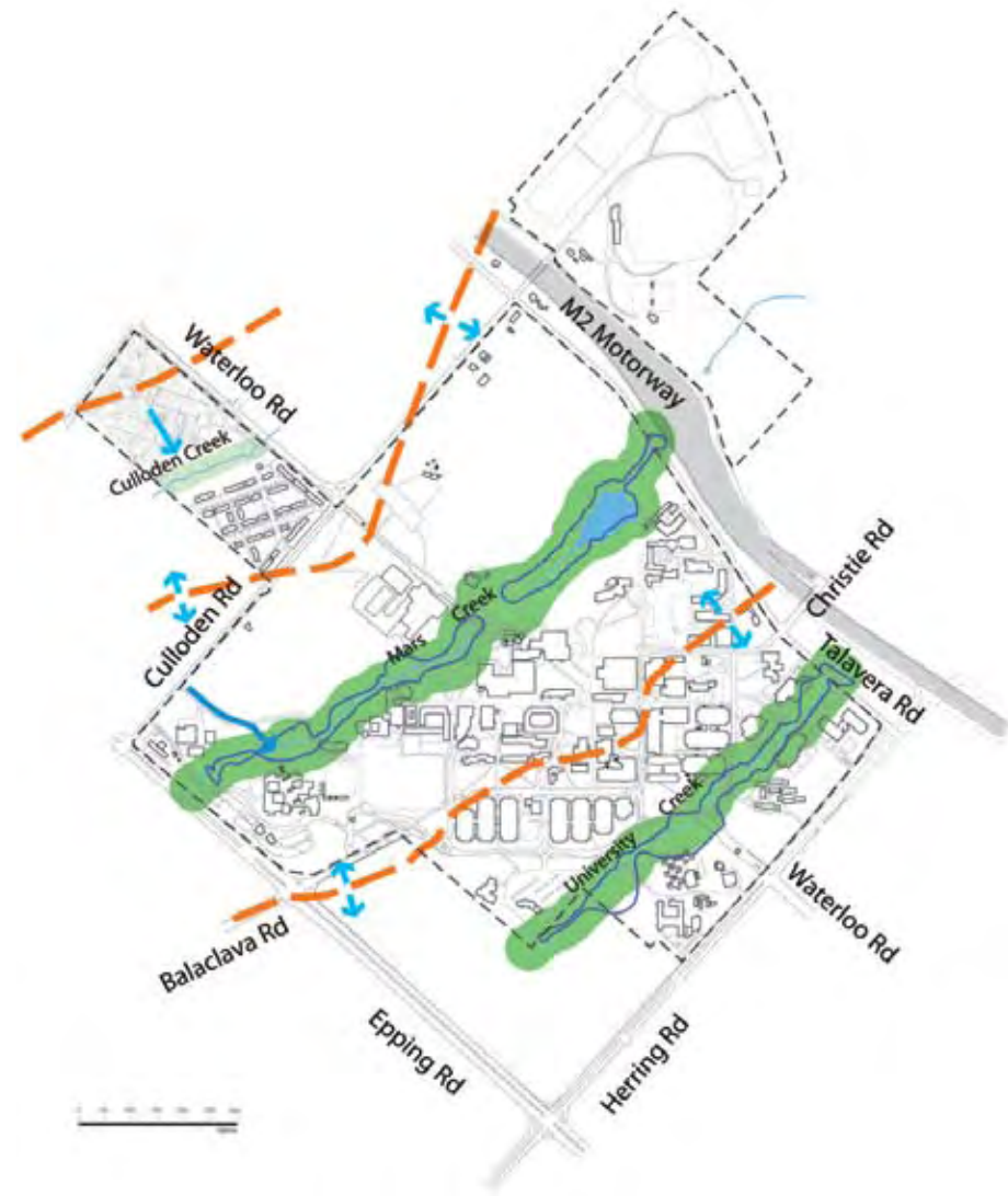
Figure 38 – Existing drainage – overland flow
