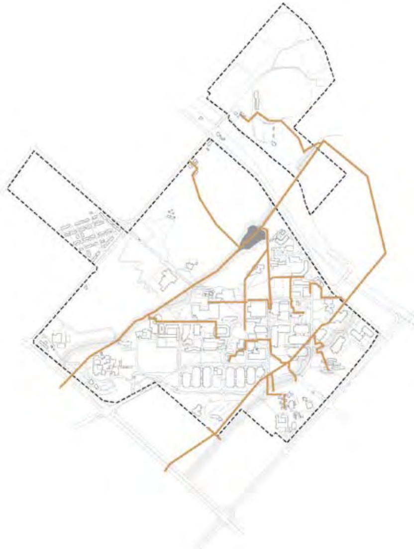
Figure 35 – Sewer trunk mains
