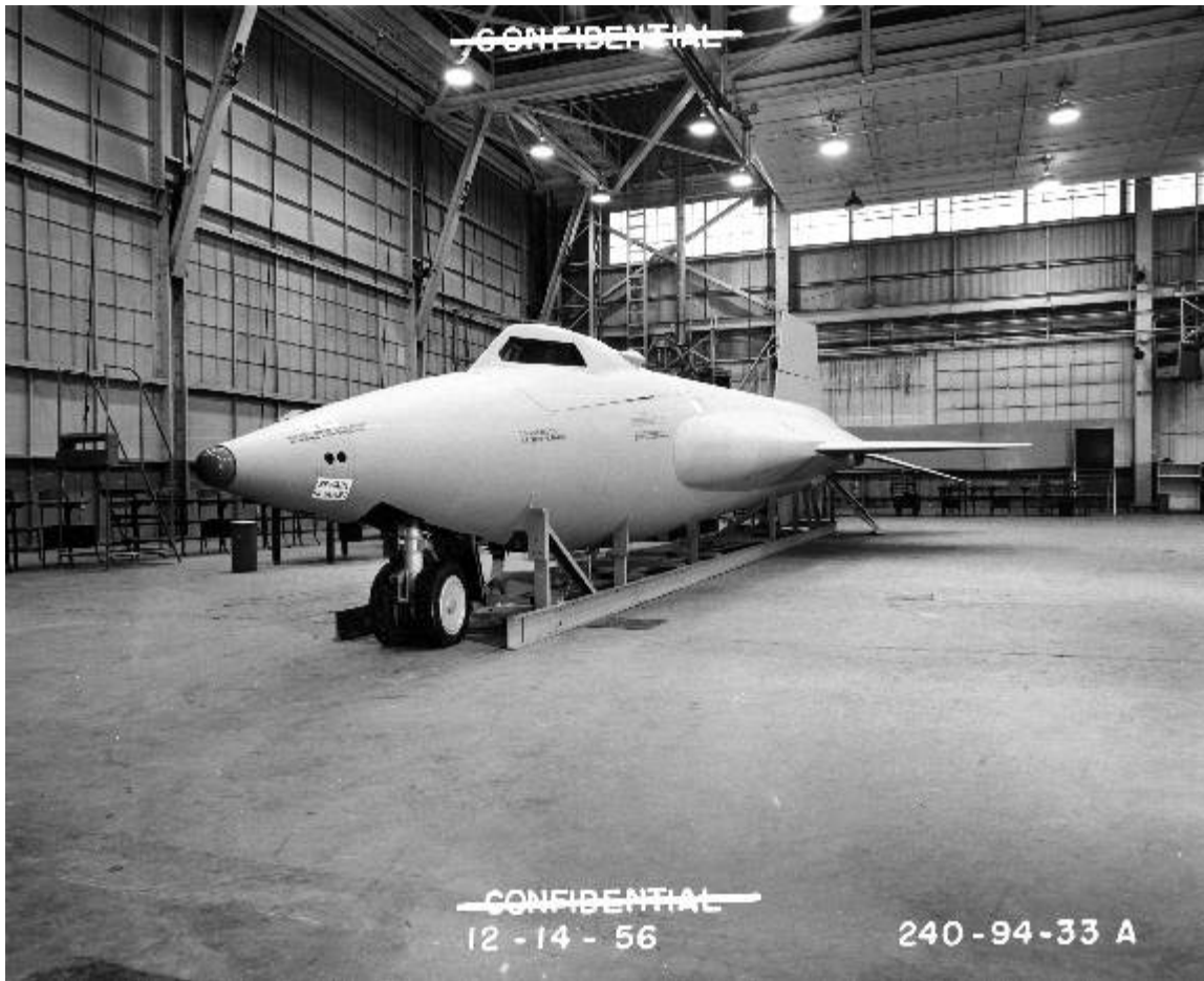
The X-15 mockup as it was inspected in December 1956. At this point, the airplane looked substantially as it would in final form with short fuselage tunnels and shorter vertical surfaces. This inspection cleared the way for North American to produce the final manufacturing drawings and begin to cut metal. (U.S. Air Force)
