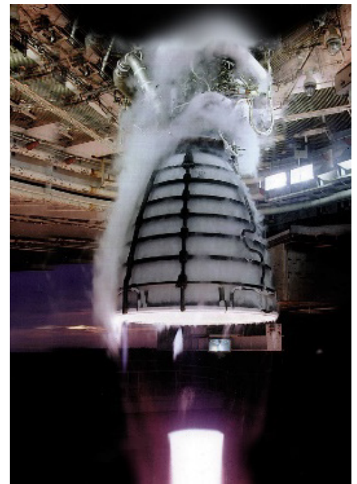
RS-25 engine undergoing a hot-fire test. (NASA)
