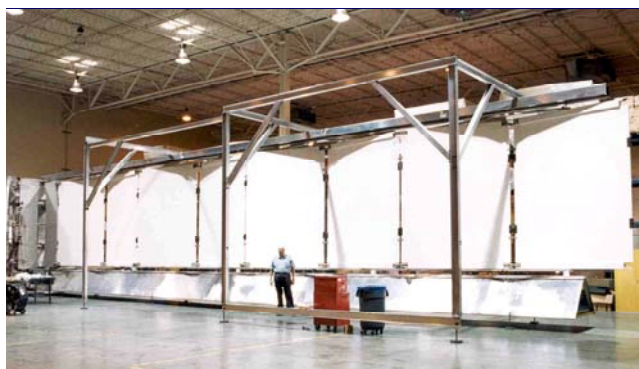
Heat Rejection System (HRS) Radiator during deployment testing at Lockheed Martin Missiles and Fire Control.
