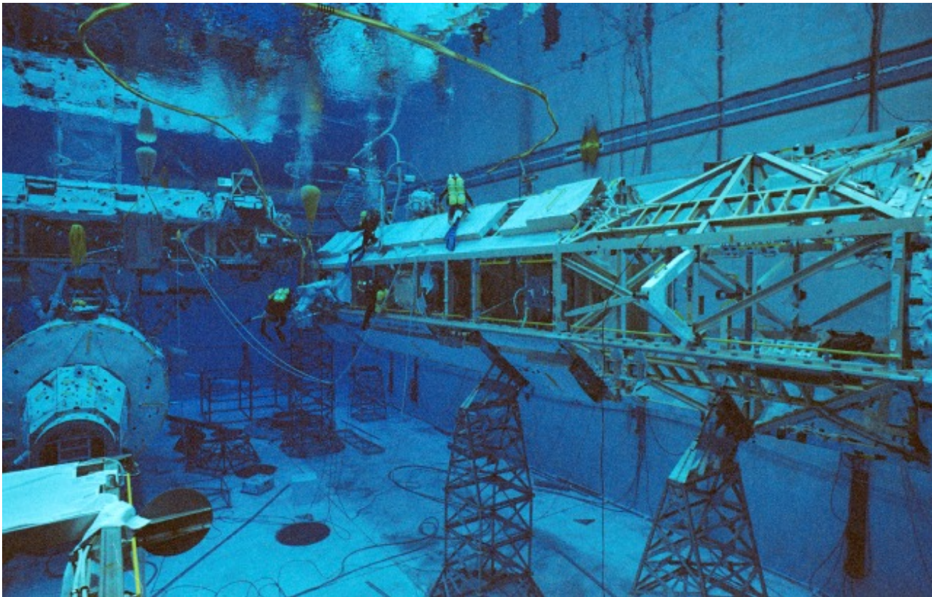
Astronauts Robert L. Curbeam, Jr. and Christer Fuglesang, STS-116 mission specialists, wearing training versions of the Extravehicular Mobility Unit (EMU) spacesuit, participate in an underwater simulation of extravehicular activity (EVA). Curbeam and Fuglesang are dwarfed by station truss segments in this overall view of the simulation conducted in the Neutral Buoyancy Laboratory (NBL) near the Johnson Space Center.
