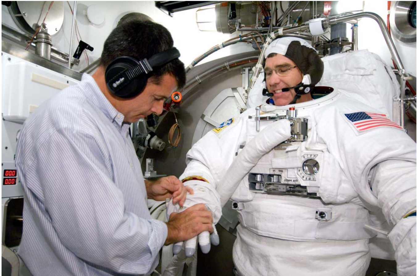
Astronaut Steve Bowen, STS-126 mission specialist, participates in an Extravehicular Mobility Unit (EMU) spacesuit fit check in the Space Station Airlock Test Article (SSATA) in the Crew Systems Laboratory at NASA's Johnson Space Center. Astronaut Shane Kimbrough, mission specialist, assisted Bowen.
