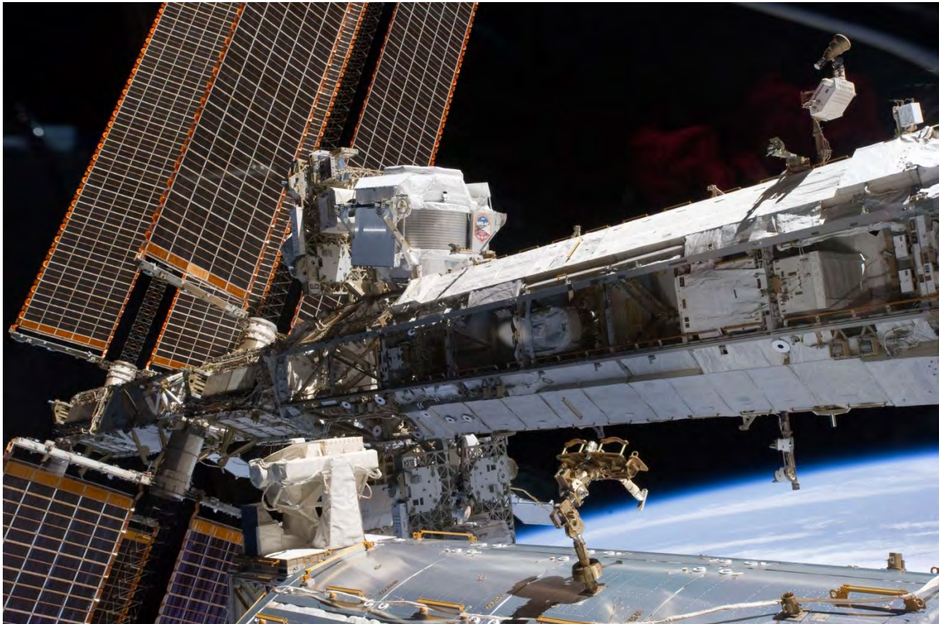
The starboard truss of the International Space Station is featured in this image with the Alpha Magnetic Spectrometer-2 (AMS) visible at center left. The AMS is collecting data at a rate of about 1.2 billion particles per month, almost double what researchers were anticipating. Photo credit: NASA
