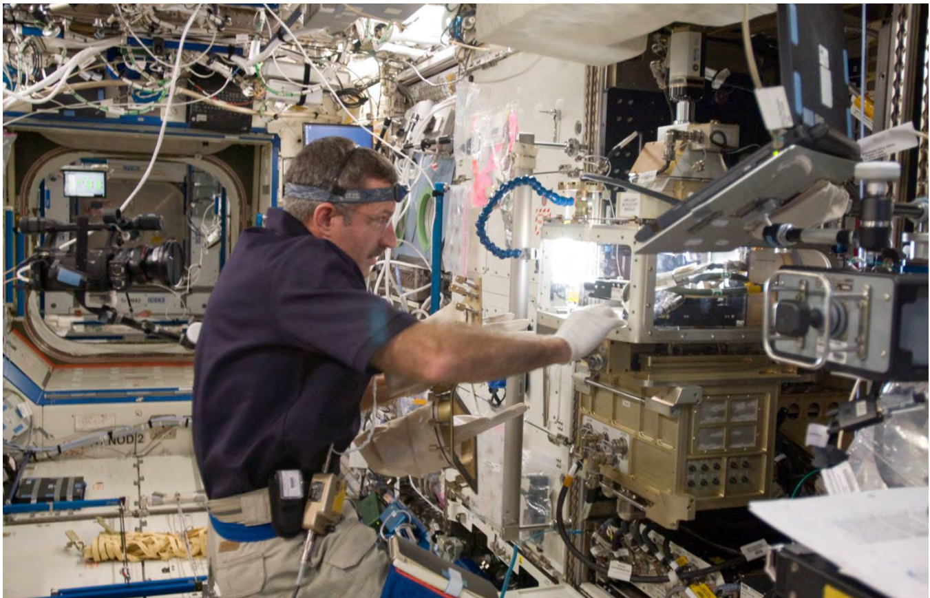
In the International Space Station's Destiny laboratory, NASA astronaut Dan Burbank, Expedition 30 commander, conducts a session with the Preliminary Advanced Colloids Experiment (PACE) at the Light Microscopy Module (LMM) in the Fluids Integrated Rack / Fluids Combustion Facility (FIR/FCF). PACE is a pre-cursor to the ACE-1 investigation. Photo credit: NASA
