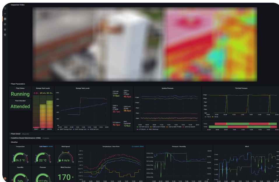
Dashboard of information gathered from the remote-piloted drone survey of the liquid nitrogen facility at the Langley Research Center.
