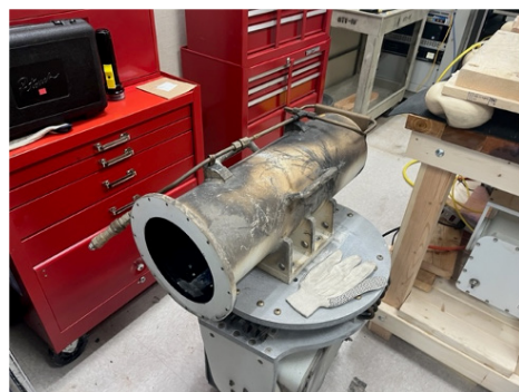
Operational Television (OTV) cameras were used before, during, and after the launch of Artemis I at Kennedy Space Center (KSC). The OTV system provided imagery acquisition, processing, recording, and distribution from the launch area during liftoff. Heat damage from the launch can be seen on the OTV camera.
