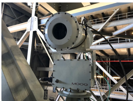
Operational Television (OTV) cameras were used before, during, and after the launch of Artemis I at Kennedy Space Center (KSC). The OTV system provided imagery acquisition, processing, recording, and distribution from the launch area during liftoff. Heat damage from the launch can be seen on the OTV camera.
