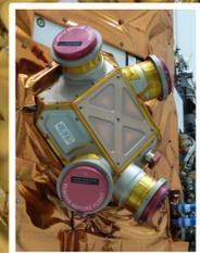
Electrospray thruster thrust is highly scalable with number of emitters.
