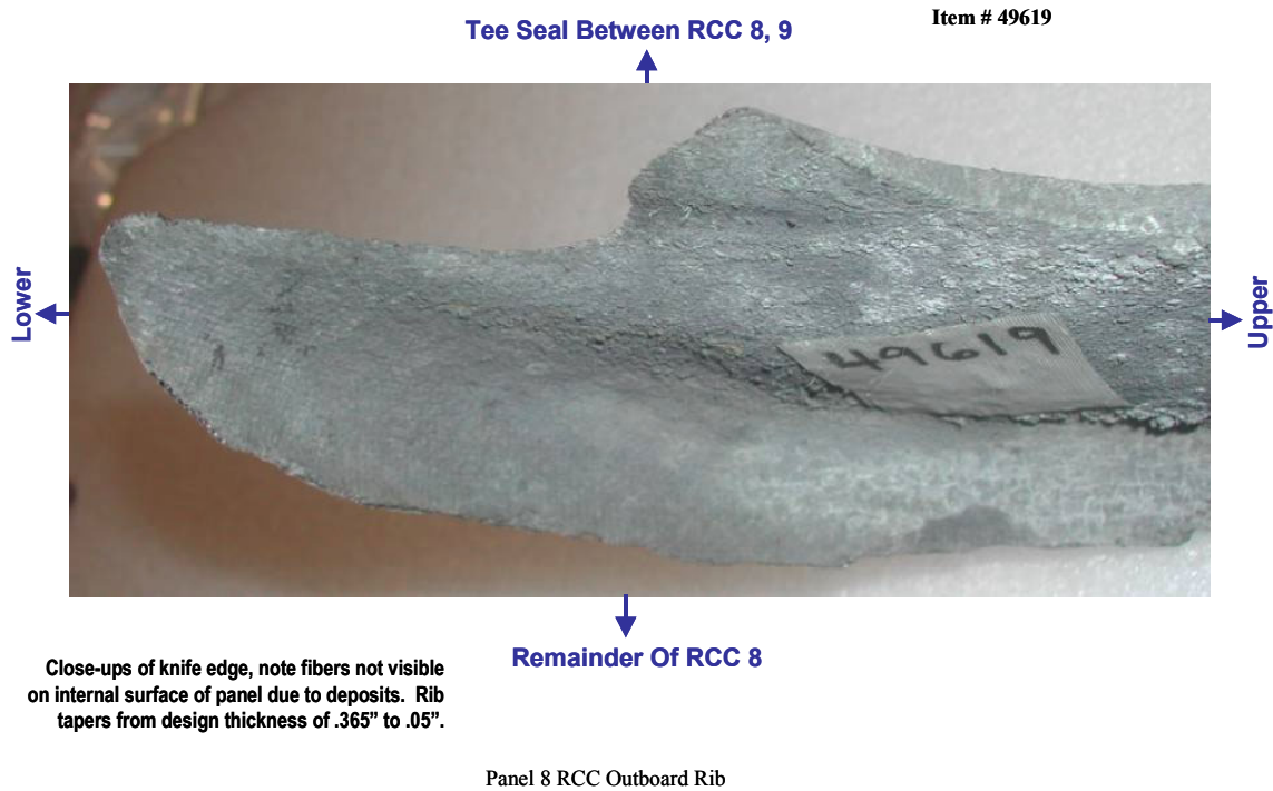
Figure 5-4. Example of rib erosion
