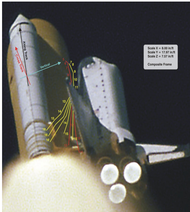
Figure 3-10. Video analysis shows impact is below wing leading edge stagnation line. Trajectories of particles are depicted after the impact.
