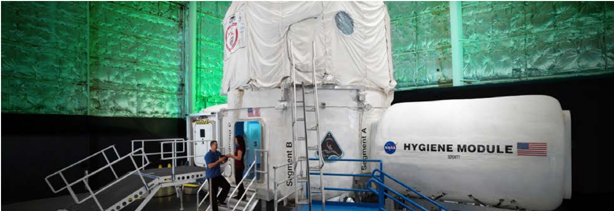
HERA is a unique 650-square-foot habitat split among two floors and a loft, designed to serve as an analog for isolation, confinement, and remote conditions in exploration scenarios.
