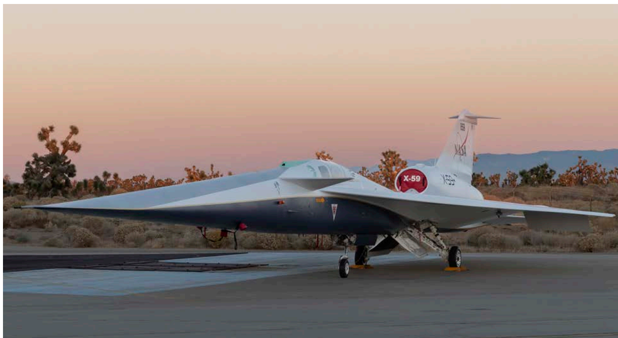
NASA's X-59 quiet supersonic research aircraft sits on the ramp at Lockheed Martin Skunk Works in Palmdale, California. The X-59 was built to demonstrate the ability to fly faster than the speed of sound while reducing the typically loud sonic boom.
