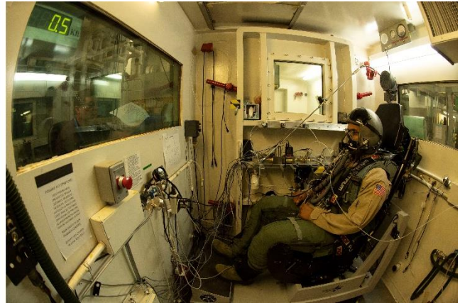
A low pressure (hyperbaric) chamber is shown at NASA partner KBR's facility in San Antonio, TX. A military test volunteer is helping verify the life support system for the X-59.
