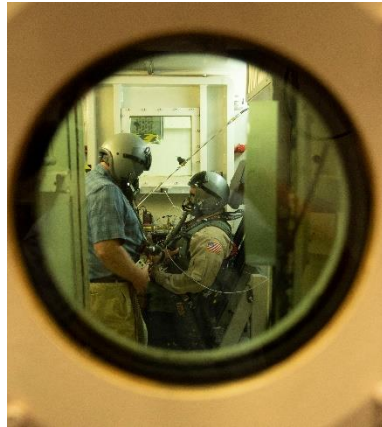
A low pressure (hyperbaric) chamber is shown at NASA partner KBR's facility in San Antonio, TX. A military test volunteer is helping verify the life support system for the X-59.
