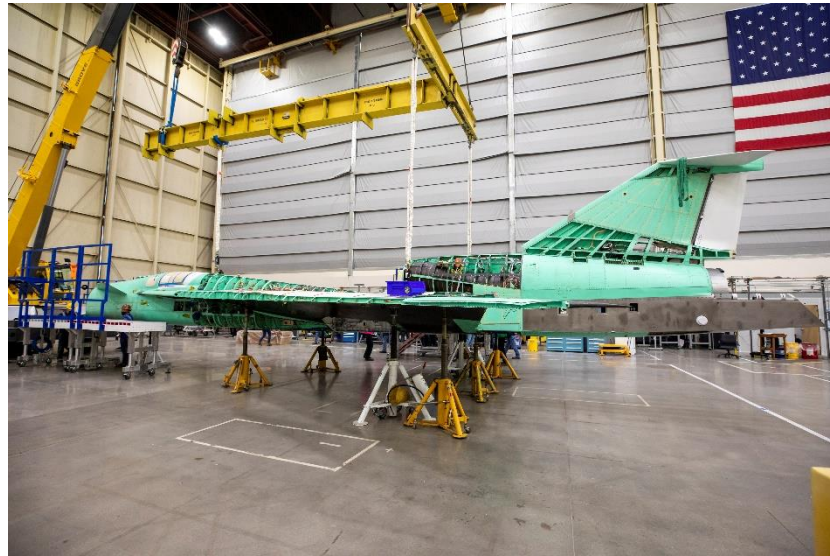
A view of the X-59 removed from the “jig” and being supported by ground supports in preparation for installation of the landing gear and other hardware required for structural testing. Image Credit: Lockheed Martin
