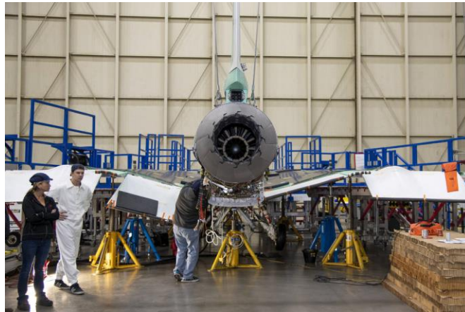
A GE Aviation F414 GE-100 engine is installed in NASA's Quiet supersonic X-59 aircraft at Lockheed martin's Skunk Works facility in Palmdale, CA. The 13-foot-long engine packs 22,000 pounds of propulsion energy and will power the X-59 to speeds up to Mach 1.4. Photo credit: NASA/Carla Thomas
