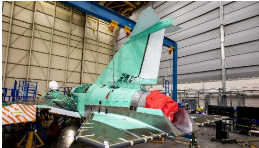
In April of 2023, the lower empennage or tail section of the X-59 was installed.
